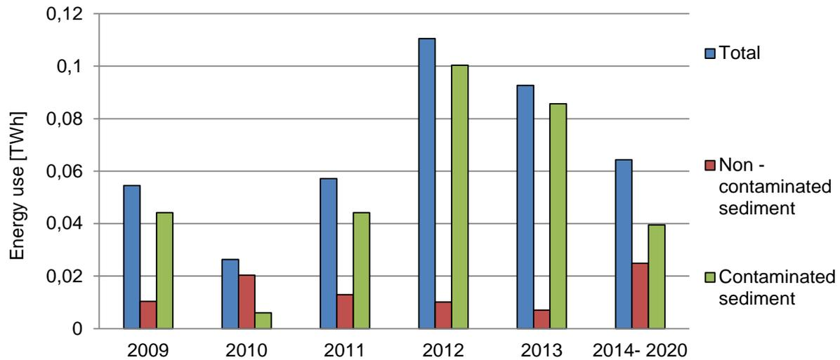
Figure 2.4: Annual energy use based on a scenario where non-contaminated sediments was disposed at sea and contaminated sediments was s/s treated.
