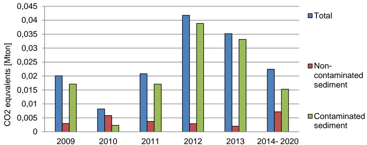
Figure 2.5: Annual CO<sub>2</sub> emissions based on a scenario where non-contaminated sediments was disposed at sea and contaminated sediments was s/s treated.
