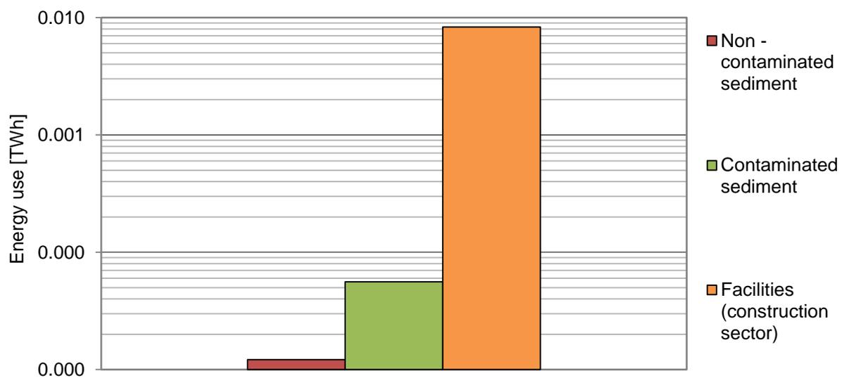
*Figure 2.7: Annual energy use for management of sediments in Sweden and for the facilities work in the Swedish construction sector.*
