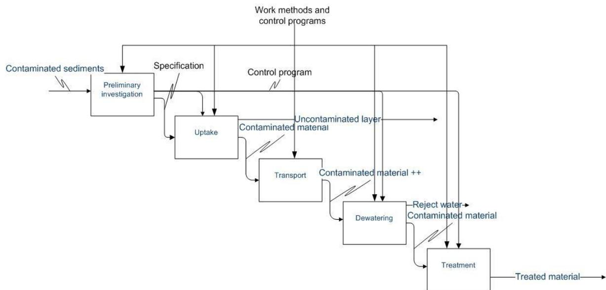
Figure 1. The many steps of a dredging operation.
