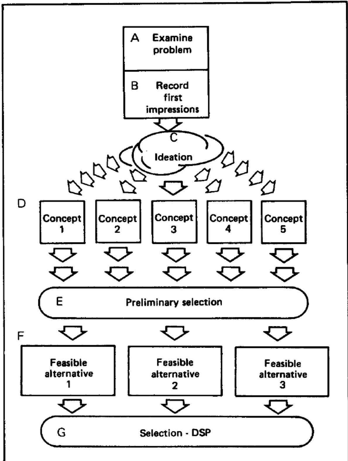
Figure 2. The process of concept selection, (Kuppuraju, 1985).
